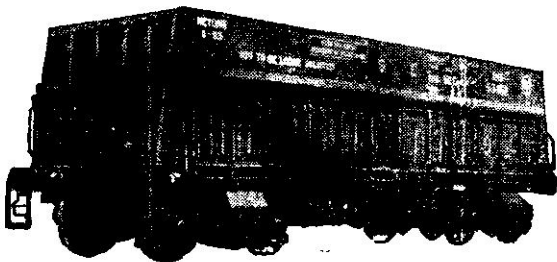
Self Discharging Mineral Wagon 'BOBS' Type - 60 ton capacity fitted with Roller Bearings and Automatic Couplers
